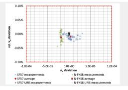
**Fig.9:** Reproducibility of V-block refractometer. Red box indicates the tolerance step. In order to give an impression of the deviation size we added the tolerance range of SCHOTT's best commercially available quality step 0.5 (red dashed line).
