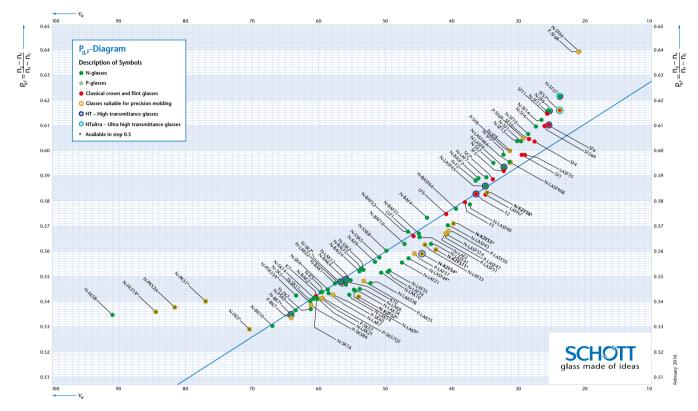
Fig. 2: P<sub>aF</sub> as a function of the Abbe number for SCHOTT's optical glass assortment. Additionally the normal line is given.
