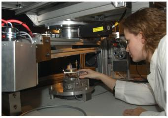
Fig. 8: Automated spectral goniometer.
