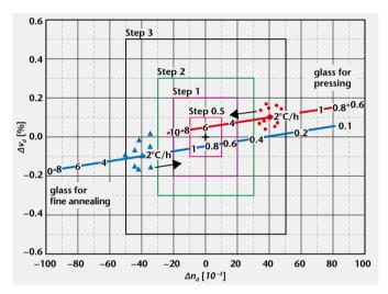
**Fig. 5:** The influence of the annealing rate on the refractive index and Abbe number of SCHOTT N-BK7<sup>®</sup> for different initial refractive indices.
