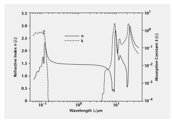
Fig. 1: Measured optical constants of fused silica (SiO<sub>2</sub> glass) [1].
