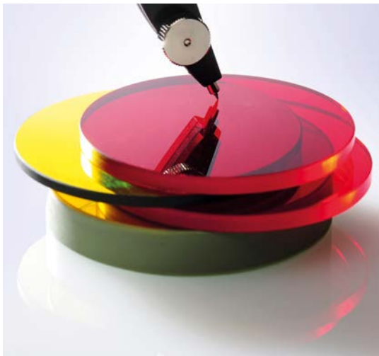
Strengthened filter glass with scratch-resistant coating.
