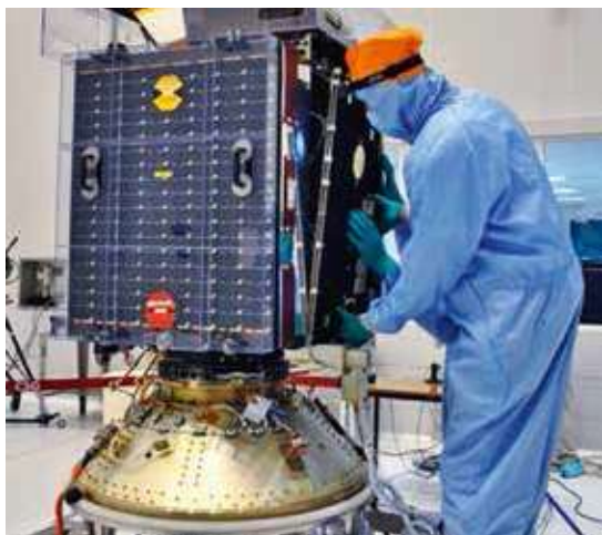
The satellite is equipped with a gallium nitride amplifier within its communication system for transmitting photos taken to earth at a height of roughly 800 km.
