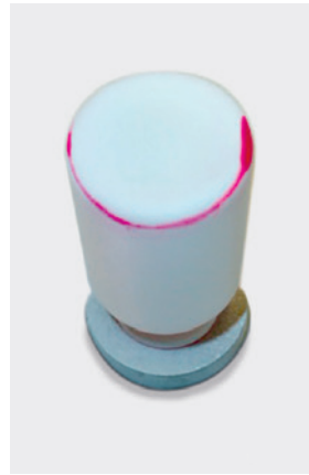
Dye penetration testing concerning glass container integrity
