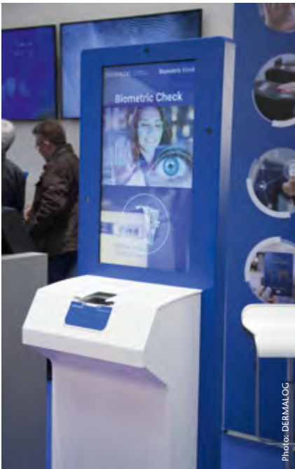
DERMALOG scanner at CeBIT 2017: on the same scan area it can read fingerprints as well as electronic passports.
