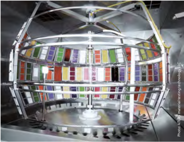
Simulated environment: The xenon lamp is encased in a tubular filter (center). Over one hundred samples can be mounted on the sample rack inside the test chamber. Temperature and humidity can also be adjusted quite accurately.
