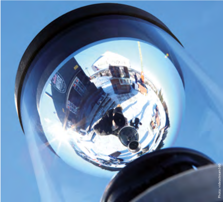
The panorama mirror delivers circular, 360-degree moving images that are recorded by a camera and then equalized by using a patented procedure. The DURAN® glass that surrounds it protects the device from scratches, environmental influences and reflections.
