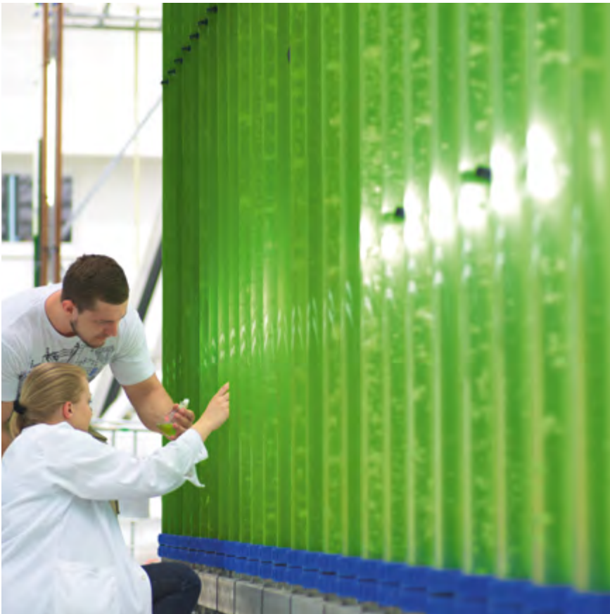
By using high-quality, round DURAN® glass tubing from SCHOTT, the light that algae need for photosynthesis can be put to better use in photobioreactors. Tubes and multiple distributors are also ideally suited for constructing state-of-the-art vertical photobioreactors.
