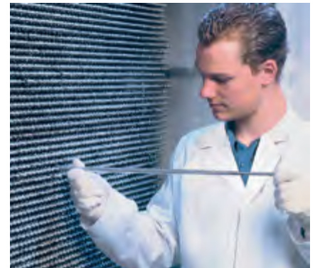
Three separate generators each with some 21,000 DURAN® glass tubes – 10,324 at each end – were installed in the world's largest ozone production system at VCP in Brazil. The outer and inner diameters of the special glass tubing required for the construction of the electrodes have an extremely narrow range of permissible variation.
