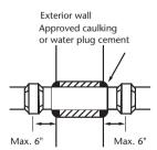
To pitch a line, snug coupling, cock joint as required to a maximum 4° deflection.
