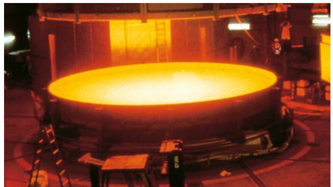
8.2-m telescope mirror blank, ZERODUR® glass-ceramic
