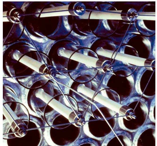
Close-up of the front of an ozonizer, inside
