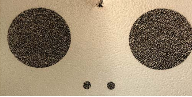
Fragmentation test for a tempered glass
