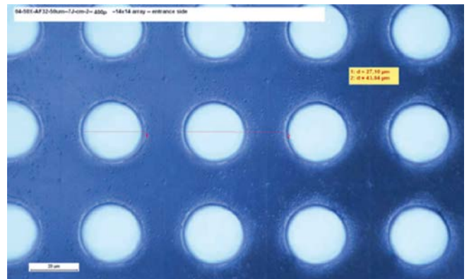
TGV technology with SCHOTT AF 32® eco 100 µm ultra-thin glass processed by excimer laser at 193 nm wavelength
