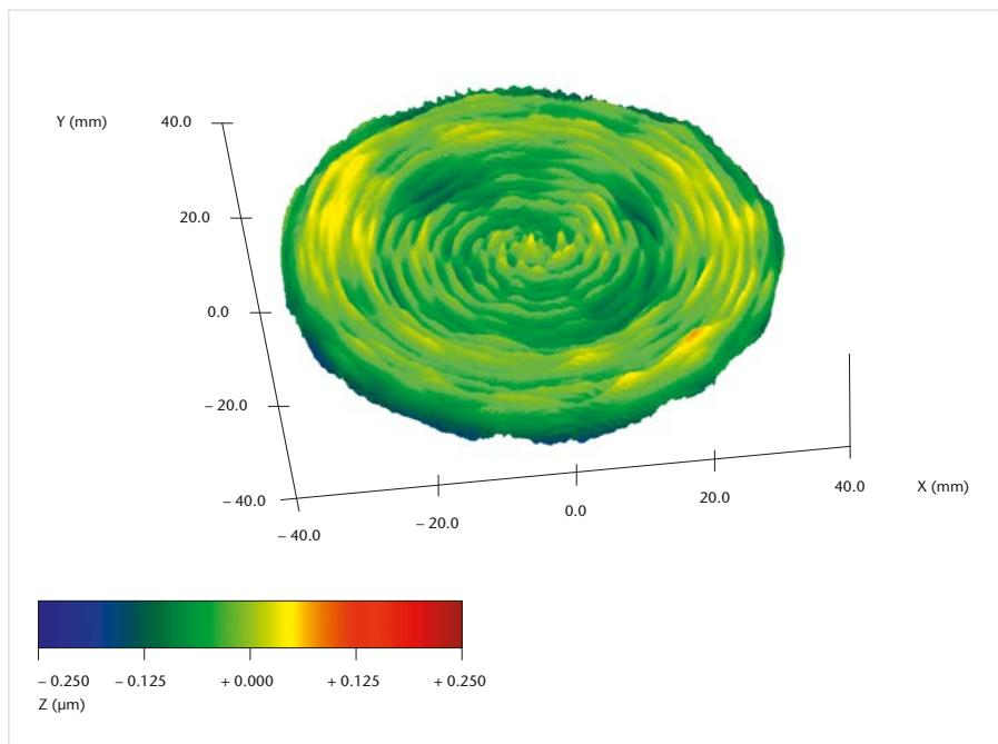
Excellent slope error performances: maximum slope error < 0.15 mrad/mm
