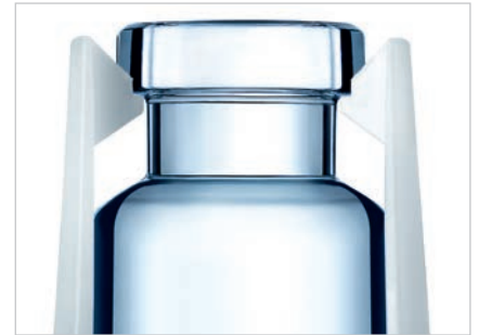
Nest with unique support for the vials, that keeps the vial bottom accessible for handling as well as nested lyophilization and minimizes glass-to-glass contact
