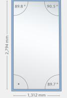
Drawing: Model panes as insulating glass with four different angles.
