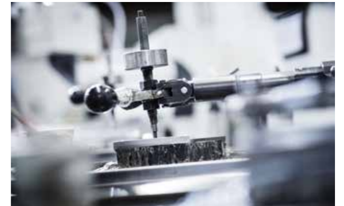
With the highest precision – polishing a lens made of BOROFLOAT®.
