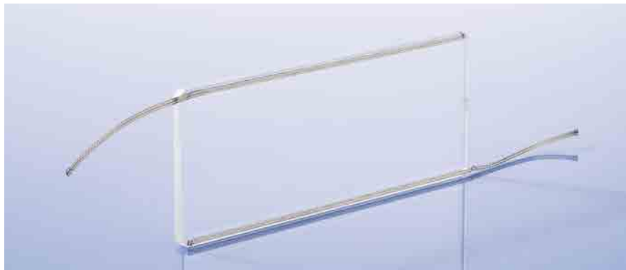
Coated glass with a transparent conducting oxide, which is both transparent and electrically conducting.
