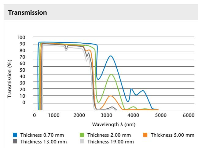
BOROFLOAT® specialty glass uses only the purest raw materials resulting in extremely low (~90 ppm) iron impurity levels and hence exceptionally high transmission values. In fact BOROFLOAT® is the industrial glass with the lowest level of iron impurity of all float glass materials in the market.
