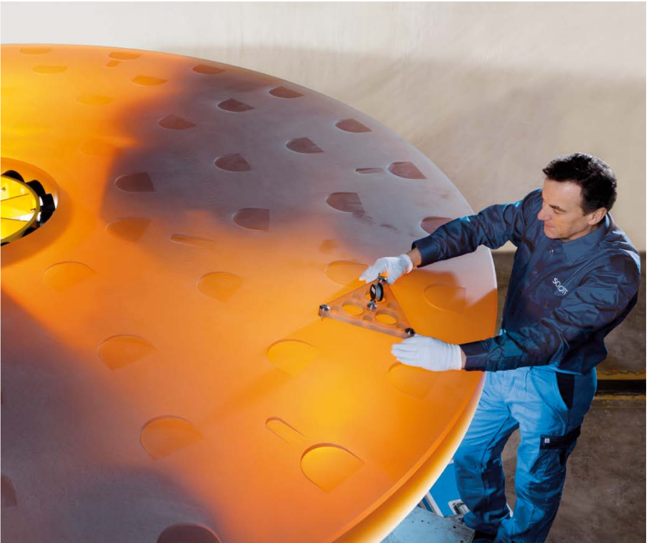
Figure 5.1 The structured rear surface of the 3.7 m primary mirror blank of the ARIES Telescope
