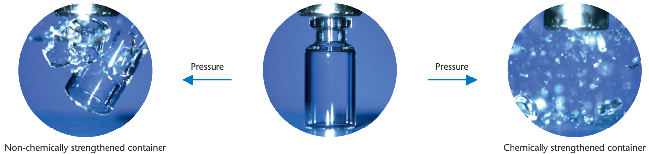
Figure 2 Breakage behavior of a non-strengthened (left) and chemically strengthened (right) glass container upon axial compression acc. to DIN EN ISO 8113 (Glass containers – Resistance to vertical load — Test method ISO 8113:2004)
