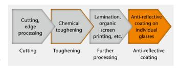
The difference using CONTURAN®. The anti-reflective glass from SCHOTT is the only one of its kind which permits chemical toughening through to the anti-reflective coating. This provides notable improvements compared to standard procedures.
