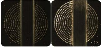
In a cleaning test, CONTURAN® DARO (left) took on a standard antireflective glass (right). For standard type staining, the SCHOTT product appeared less dirty from the outset and required just three swipes to regain full cleanliness. In contrast, the comparison product showed clearly more traces of staining and remained unclean after three swipes.
