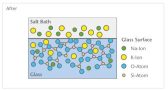
The ion exchange at the glass surface generally involves sodium ions being replaced by potassium ions. This increases compressive pressures which deter cracks in the glass.
