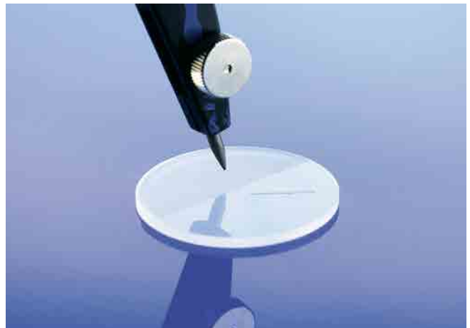
A partly coated disc: a scratch-resistant AR coating (upper left) and an uncoated surface (lower right).
