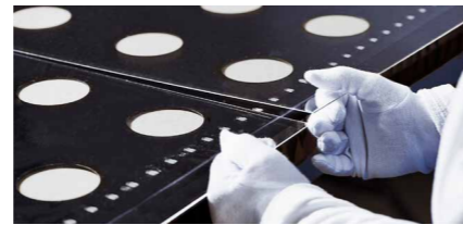
Breaking the glass at defined edge
