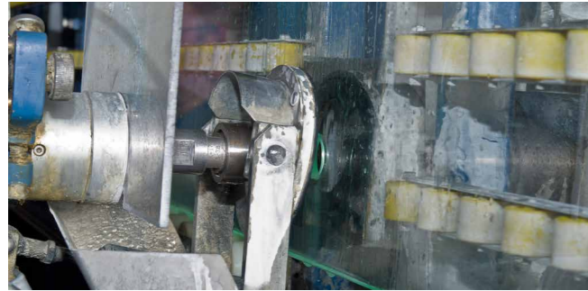
Drilling on both sides with a horizontal drilling machine
