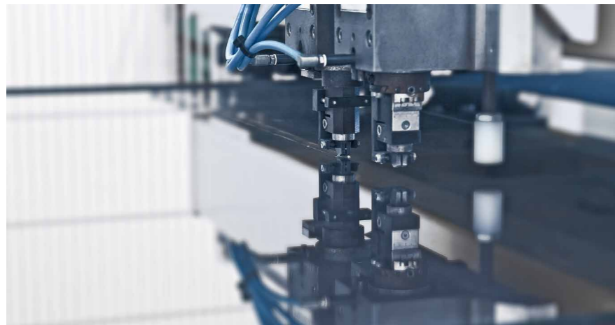
Scoring the glass with cutting wheel
