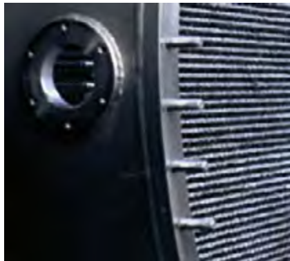
Three separate generators each with some 21,000 DURAN® glass tubes – 10,324 at each end – were installed in the world's largest ozone production system at VCP in Brazil. The outer and inner diameters of the special glass tubing required for the construction of the electrodes have an extremely narrow range of permissible variation.
