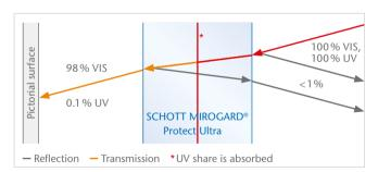
MIROGARD® Protect Ultra absorbs almost 100% of harmful UV light. Nevertheless, it still transmits nearly 100% of the visible light, with no annoying reflections and with the acknowledged excellent  $R_a$  = 100 color rendering index of SCHOTT MIROGARD®.
