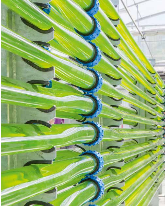
Tubular Glass Photobioreactors (PBR) located at A4F - Algae for Future, Portugal
