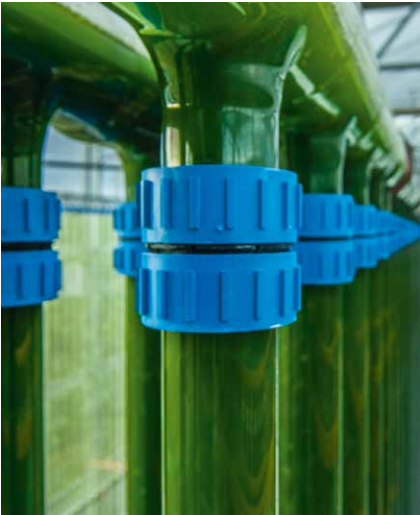
Manifolds and Couplings, Fence System, ecoduna AG © ecoduna.com
