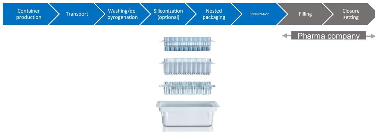
Figure 3: Process flow for processing and filling injectable drugs in RTU containers (simplified for all containers)
