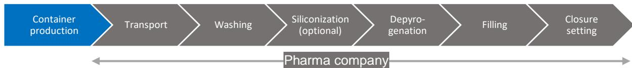
Figure 2: Process flow for processing and filling injectable drugs in bulk containers (simplified for all containers)
