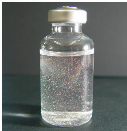
Flake-like particles by visual inspection
