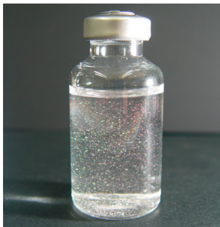
Flake-like particles by visual inspection
