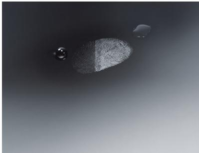
With its glass CONTURAN® DARO, SCHOTT combines an anti-reflective coating with a film that protects against dirt on the cover glasses of professional touch displays for the first time ever. This photograph shows the left half of the picture with and the right half without the DARO coating. Photo: SCHOTT.
