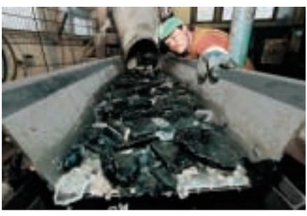
*The processing of mixed glass from picture tubes involves separation, cleaning and optical sorting.*
