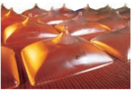
*Schott uses cullet from used picture tubes as a raw material for new funnels.*
