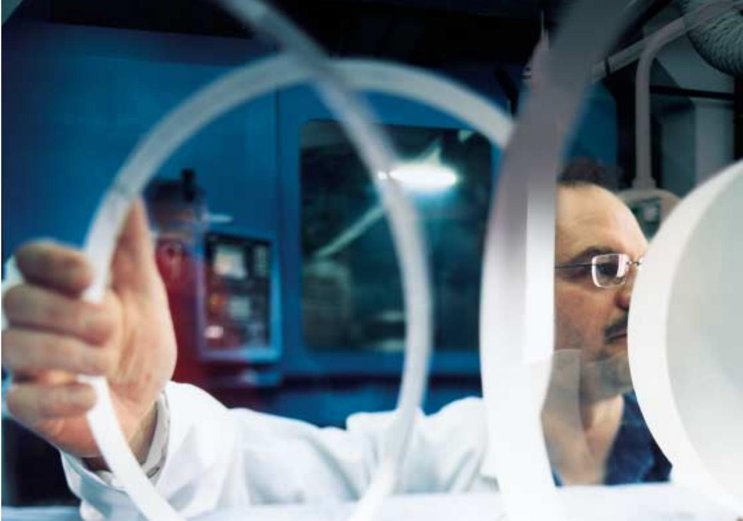
Due to its high resistance to radiation and absence of any compaction (local changes in density) when bombarded by lasers, the optical high-tech material calcium fluoride crystals are used for lens production in microlithography.
