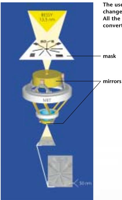
In cooperation with the Lawrence Livermore National Laboratory in California, Carl Zeiss SMT AG has developed a prototype for EUVL technology, the Micro Exposer Tool (MET), with highly precise mirrors instead of lenses. "Zerodur" from Schott is particularly well suited as a mirror substrate for this new technology because of its extremely low coefficient of thermal expansion.
