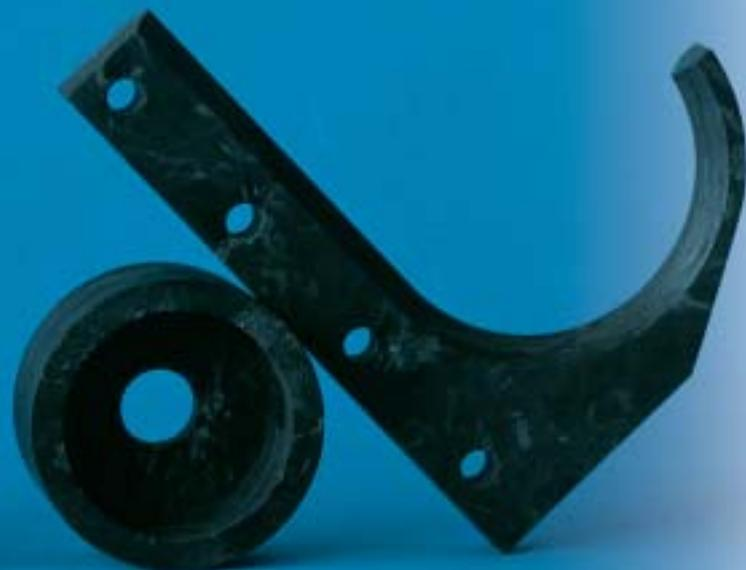
The use of matted fibers is a technological advance. Compared with manufacturing methods based on continuous fibers, composites can not only be made more economically, but also permit the production of components with other geometries because of their isotropic features.
