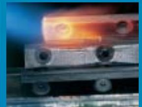
"Fortadur" has a very good breaking and flexural strength, tolerates temperatures of up to 1,200° C and can be used to produce components in complex geometries.
