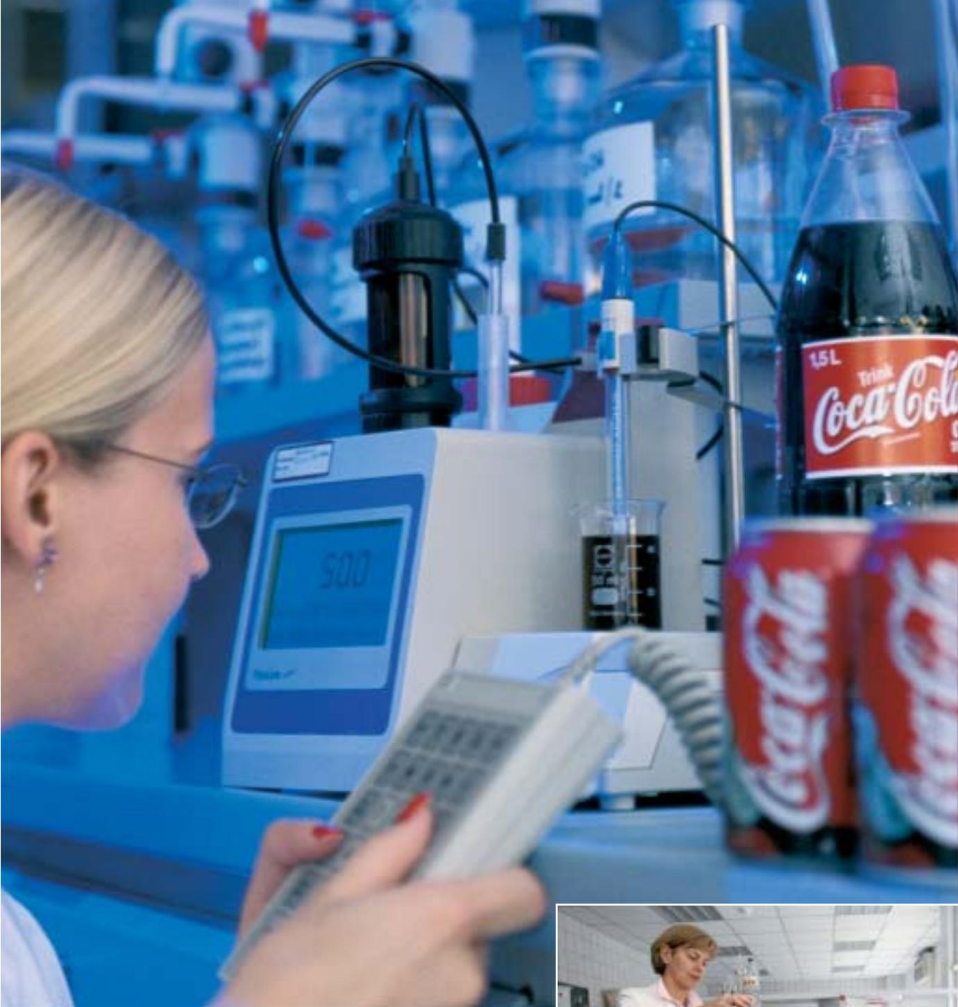
Soft drinks are subject to constant quality control. Titrators are used as analytical equipment at the production facilities of Coca-Cola's concessionaire in Liederbach. They ensure a consistent taste quality with the help of precise measurements.
