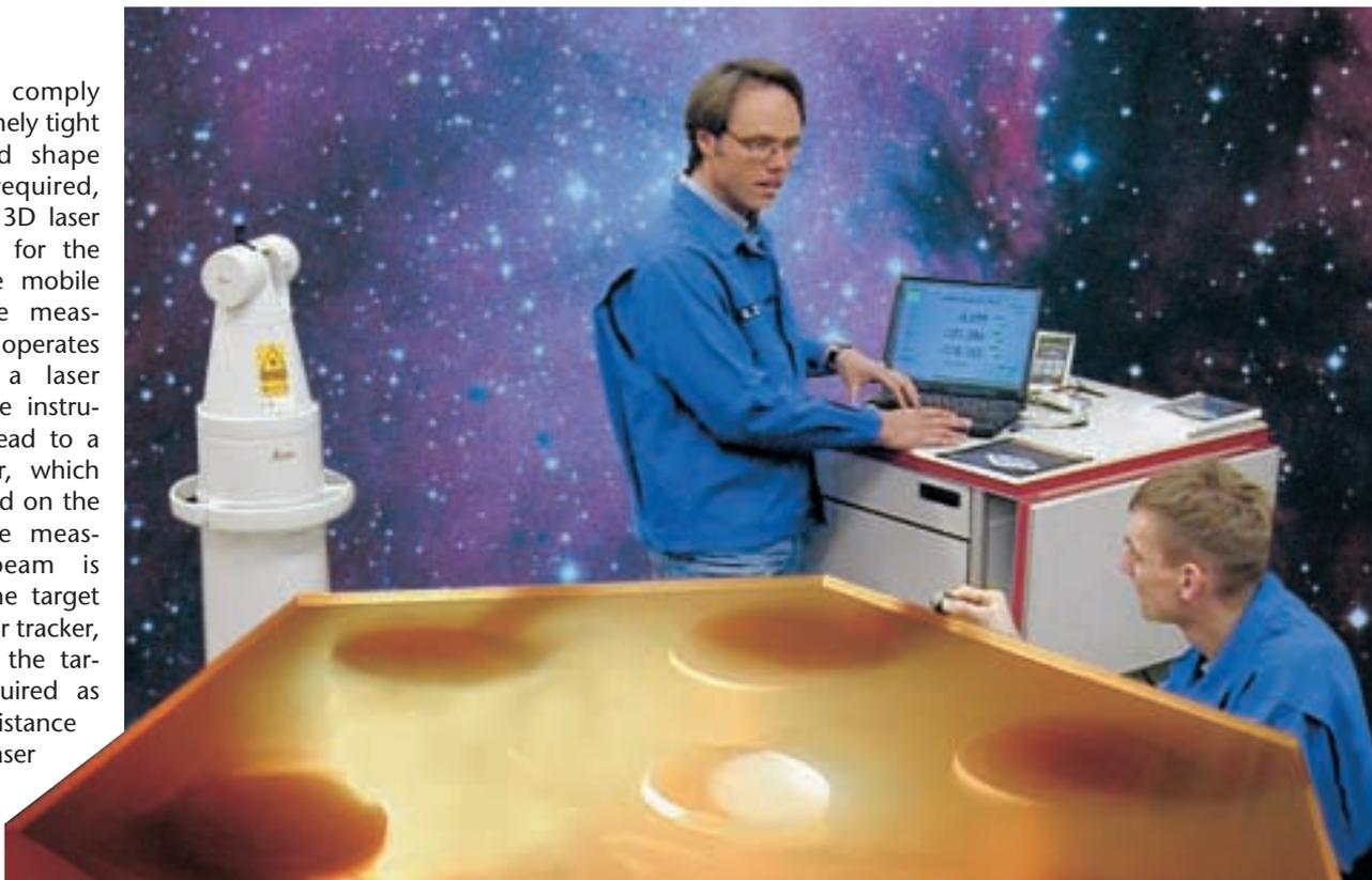
*The laser tracker provides not only high measuring accuracy, but also mobility and sophisticated inspection and evaluation methods.*
