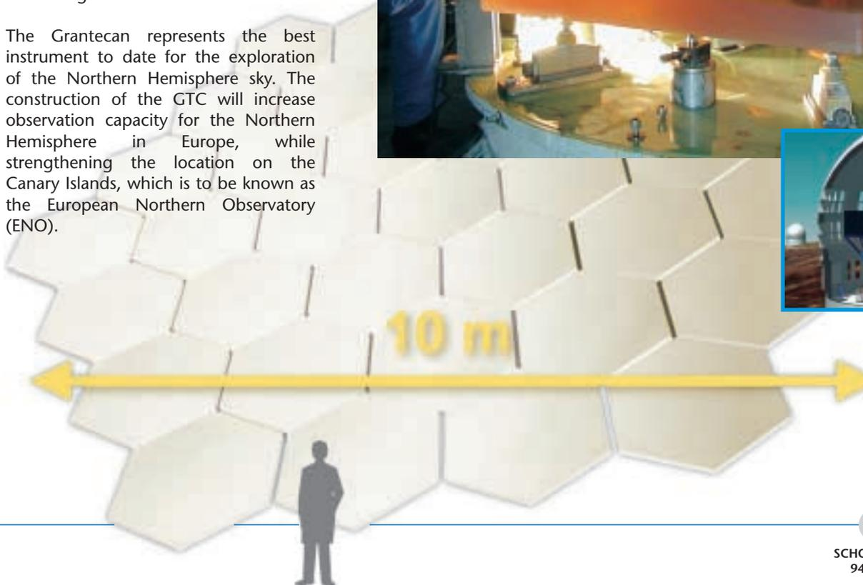
*The primary mirror is made up of 36 hexagonal segments: With a diameter of 10.4 meters and a maximum size of 11.3 meters, Grantecan is the world’s largest telescope.*
