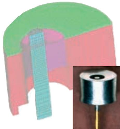
*For product optimization of airbag igniters help is provided by so-called finite-element simulation.*
