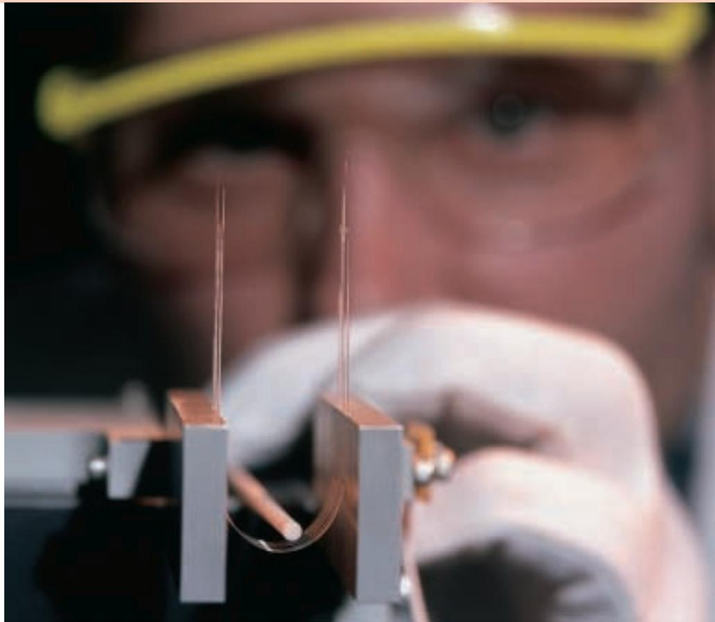
*Two-point bending test for examining the resistance of fibers to breakage.*
