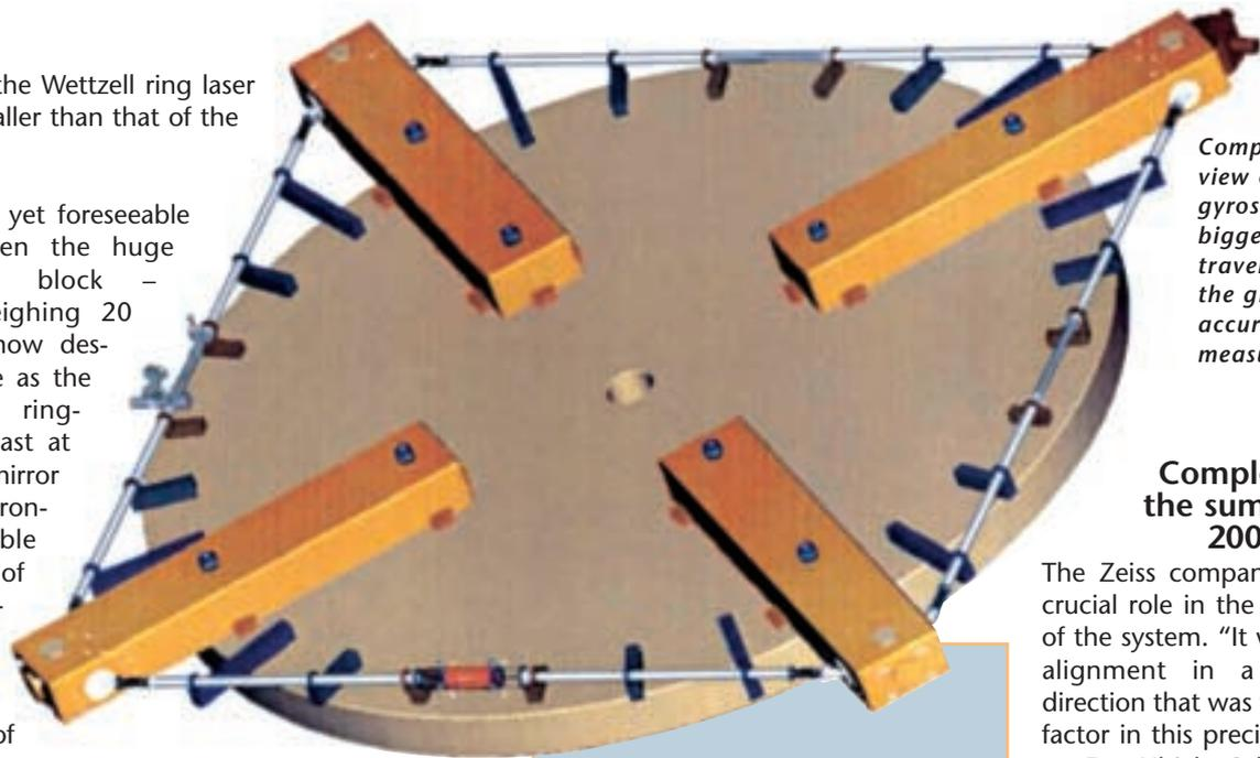
*Computer-drawn view of the laser gyroscope: the bigger the circuit traveled by the rays, the greater the accuracy of the measurements.*
