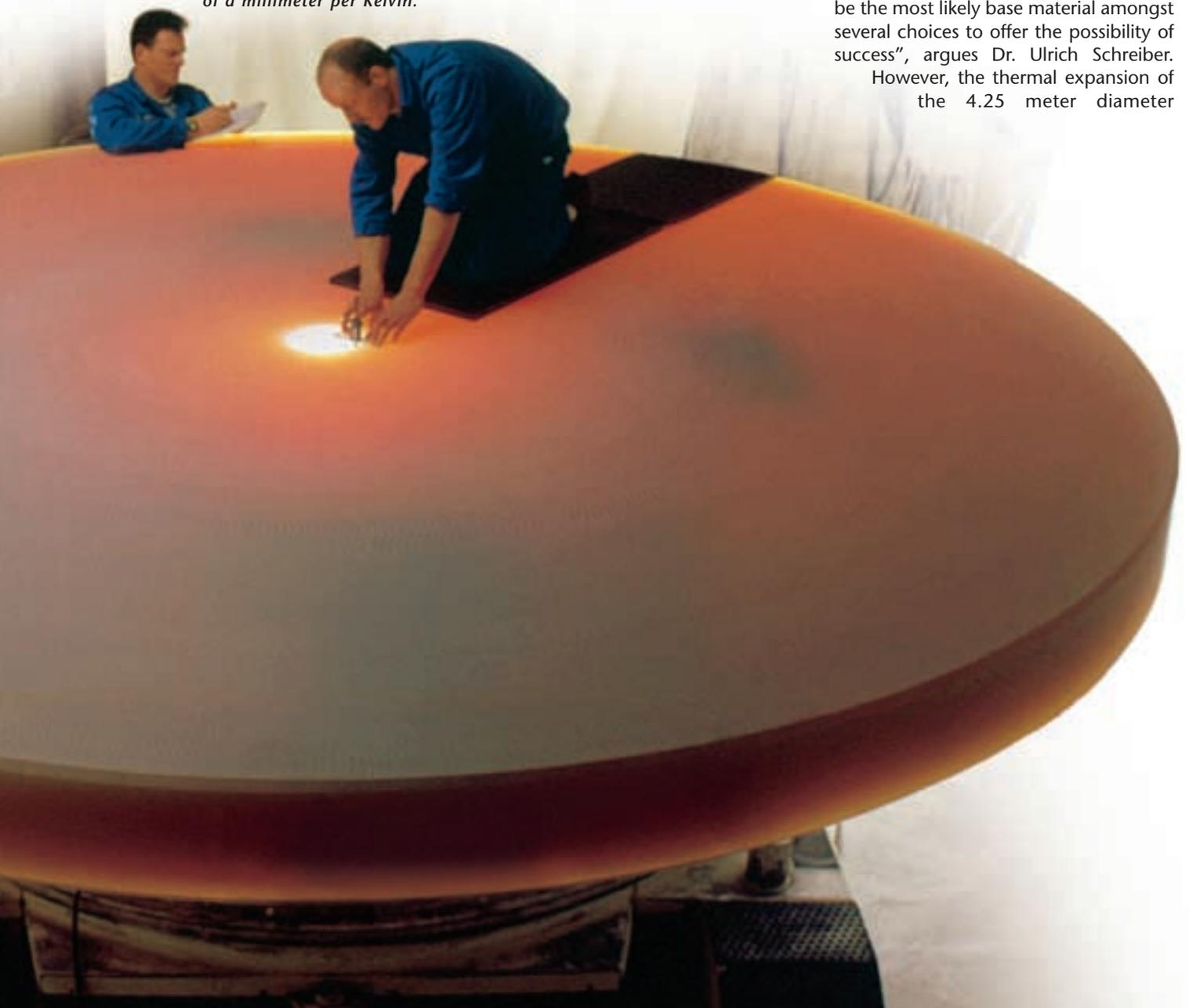
monolith for the Wettzell ring laser had to be smaller than that of the prototype.
