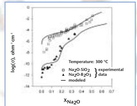
Calculated dependencies for the density and electrical conductivity in sodium silicate and sodium borate glasses together with the corresponding experimental data (from O.V. Mazurin et al., *Properties of Glasses and Glass-Forming Liquids*, Nauka, Leningrad, 1975). The precision of the modeling corresponds to the precision of the experimental measurements.
