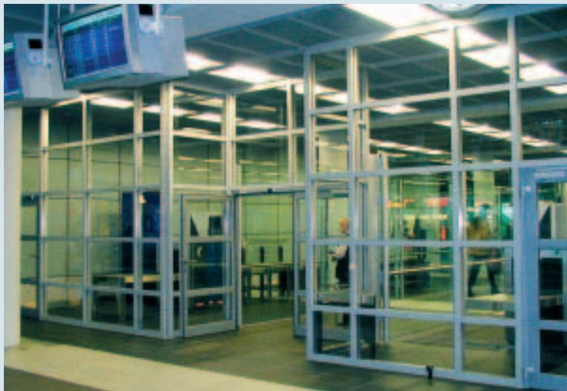
The dividing wall in front of the security gate in the departure area was made with six-millimeter thick "Pyran S" special glass supported in steel fire protection profile frame system from Schueco. The system meets the 30-minute integrity standard.
