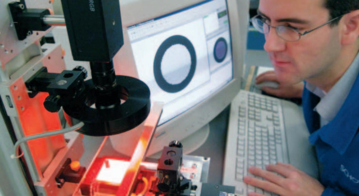
Laboratory facility for machine vision applications with CCD (Charged Couple Device) camera and ringlight. The contours of the control object are rendered visible on the monitor.
