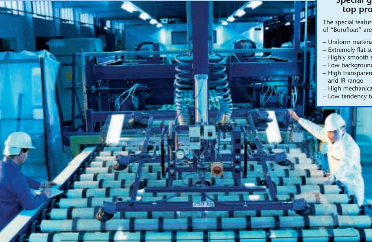
*In Jena Schott was the first to produce Borosilicate glass using the microfloat process.*
