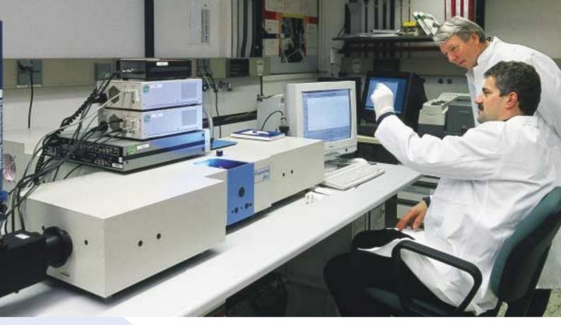
Modern measuring technology makes it possible to detect traces of individual elements in optical materials at levels of less than 50 ppb (50 parts per billion).
