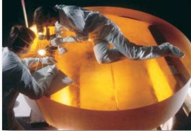
Quality control of a "Zerodur" disk: with the introduction of "Zerodur" glass ceramic, SCHOTT Glas in Mainz set a new international standard for astronomical mirror substrates from 1970 on. This engineering material is characterized by its zero thermal expansion.
