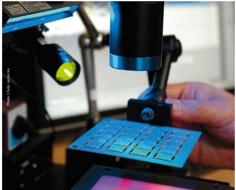
Integrated systems that feature optimized lens and lighting solutions ensure high quality standards in various areas of manufacturing, e.g. in the inspection of TFT modules or solar panels.
