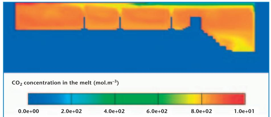
Calculated distribution of dissolved CO<sub>2</sub> in a melting tank (concentration contours in the vertical cross-section of a melting tank.)
