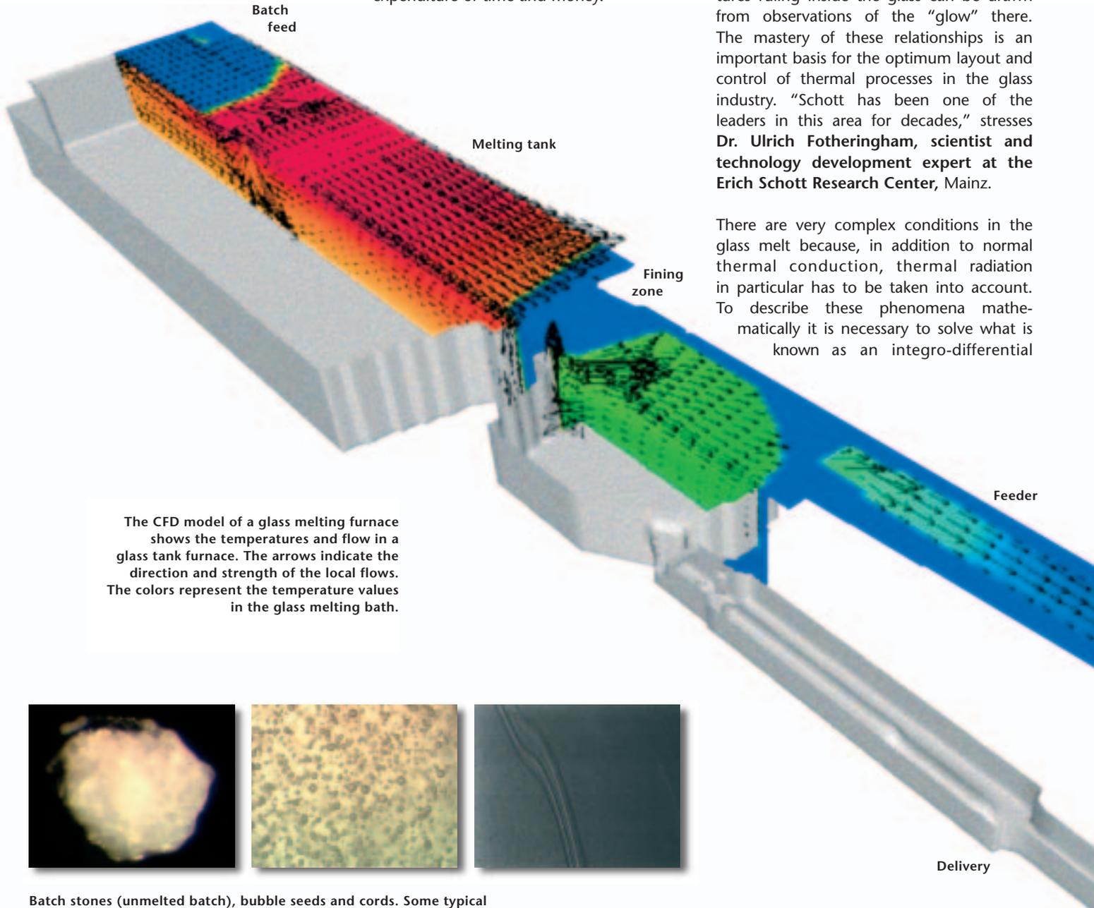
The CFD model of a glass melting furnace shows the temperatures and flow in a glass tank furnace. The arrows indicate the direction and strength of the local flows. The colors represent the temperature values in the glass melting bath.
