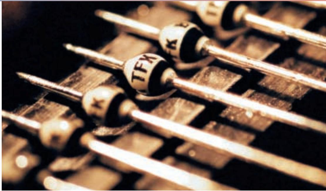
*Rectifier diodes for high voltage and high temperature applications.*
