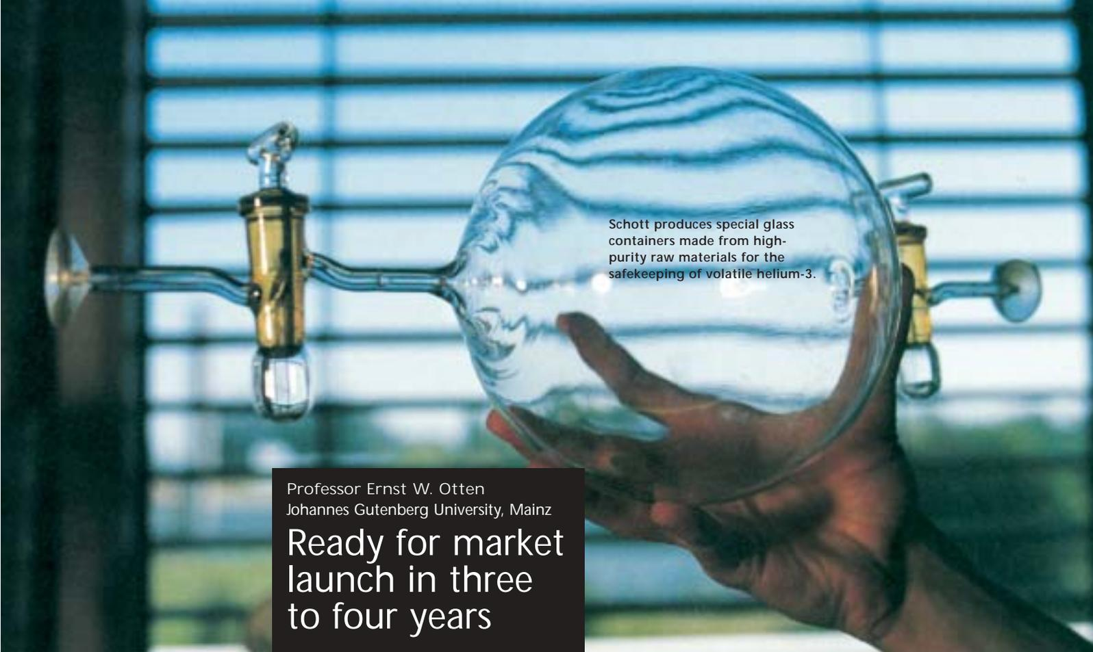
Schott produces special glass containers made from high-purity raw materials for the safekeeping of volatile helium-3.
