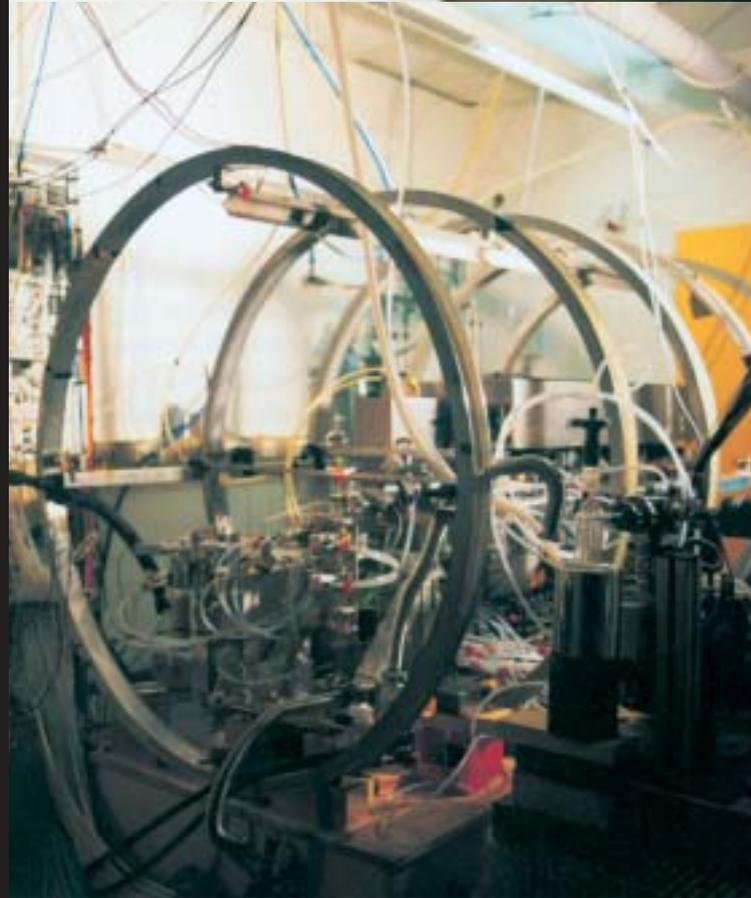
Five spools produce a magnetic field in which helium-3 is polarized with an infrared laser.
