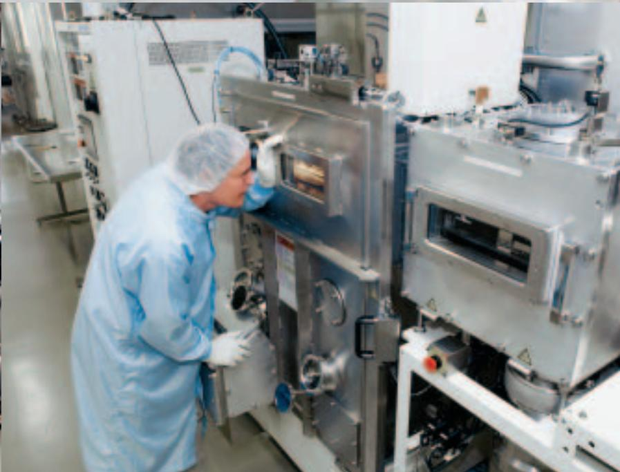
OLED components are processed in inert gas and
