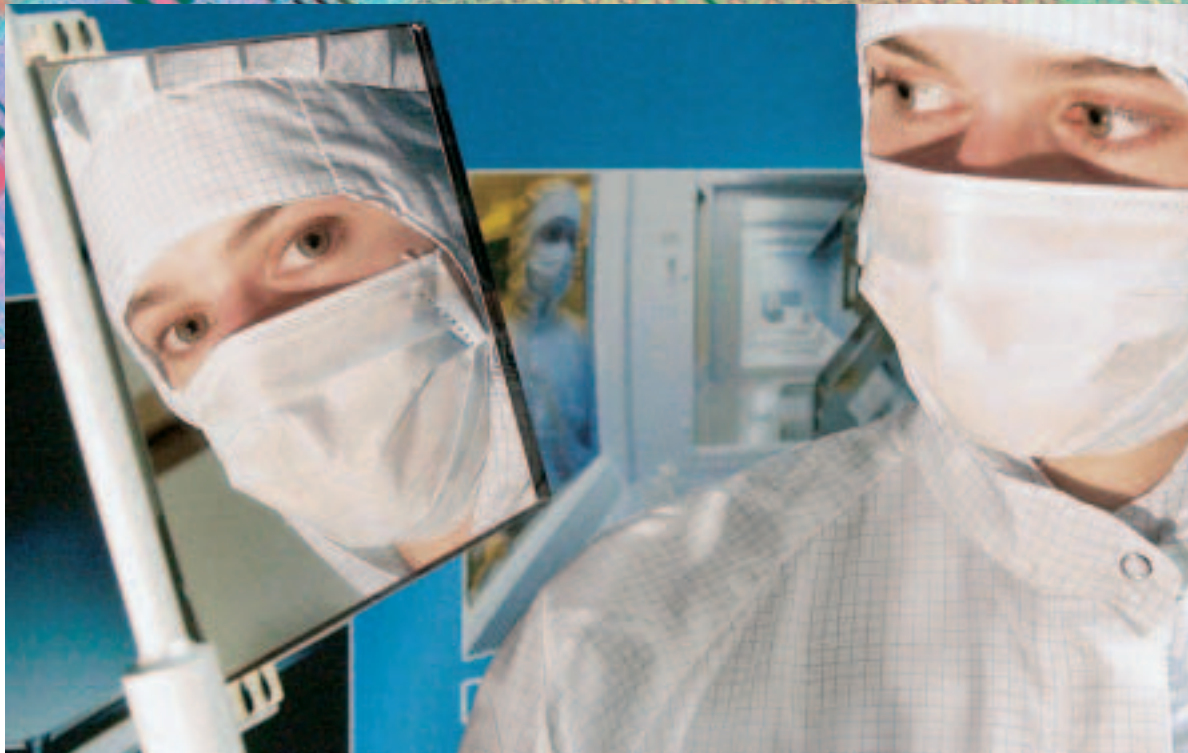
Coated mask blanks are the basis for photomasks used in wafer steppers for the manufacture of semiconductor chips.
