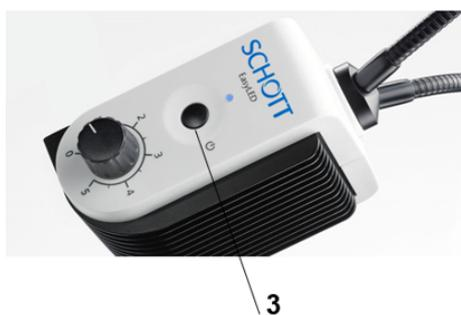
With the double Spotlight Plus lighting system you can switch between the two individual light heads by repeatedly pressing the "on" and "off" button.
