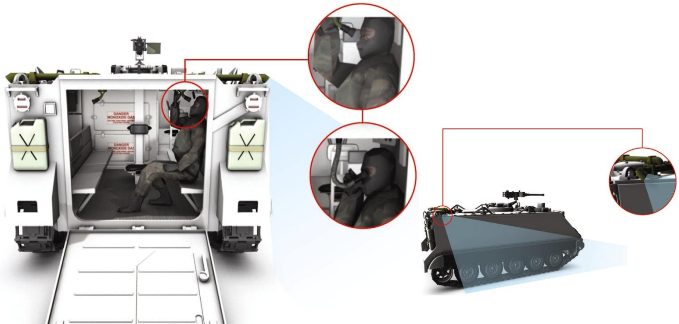
Example application of remote viewing through a SCHOTT Wound Image Bundle.
