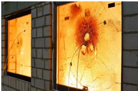
A fire test is performed for 60 minutes on a NOVOLAY® secure glass laminate that had already been shattered by shots from a gun in accordance with the DIN EN 1363 standard. Photo: SCHOTT
