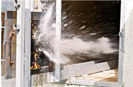
Photo shows a pane of PYRANOVA® secure that was first subjected to a fire test for 30 minutes then attacked with a 9 mm Luger army pistol. The extremely hot glass laminate from SCHOTT resists three shots fired from a 9 mm caliber gun at a speed of 400 m/s. Photo: SCHOTT:
