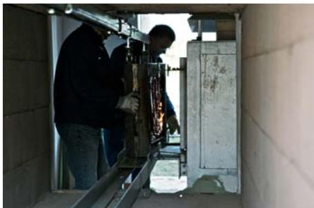
A glass laminate is subjected to either 30 minutes of fire (standard temperature curve) at a temperature of more than 800 °C or for a period of 5 minutes (simulation of a Molotov cocktail) and then bullet tested at the world's first fire and ballistic facility in Thuringia, Germany. Photo: SCHOTT
