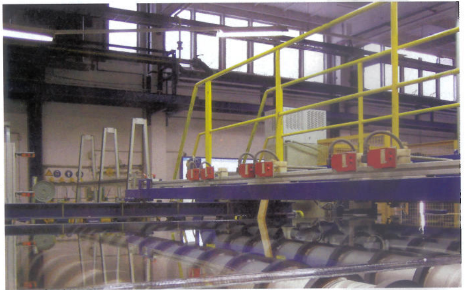
Figure 1: The smooth, distortion-free surface of Pyran Platinum floated glass-ceramic fire-rated glazing manufactured using the microfloat process at Schott Technical Glass Solutions GmbH in Jena, Germany, is evident in this photo of the formed glass ribbon.
